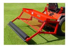
The floating roller will push back any plucked divots without closing the penetrations; the roller can be lifted out of work if required. An adjustable scraper bar is fitted to the rear of the roller.
